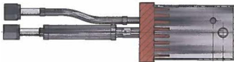
Figure 10.17, Cold Finger Fins
