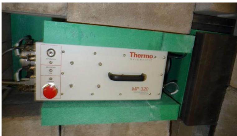
Figure 10.27, Thermo MP 320 Neutron Generator at NETL
